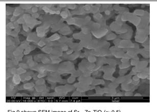
Fig 9.shows SEM image of  $Sr_{1-x}Zn_xTiO_3(x=0.5)$
